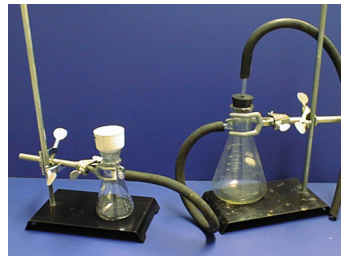
Old-School Vacuum Trap on right, connected to Buchner funnel filtration assembly. Note lack of inline filter, secondary containment. Trap requires additional ring stand and hardware for stability. Setup/cleaning process is complicated.
